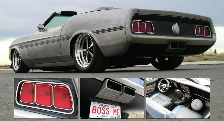
The '71's bumpers are flush fit and custom contoured to match the body while belly pans were added front and rear. The taillights were custom made by Acrylic Concepts in Calgary and blink sequentially like the taillights of it's Mercury Cougar cousin.
